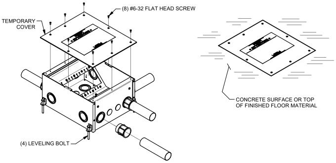
TYPICAL INSTALLATION HEIGHTS FLOOR BOX TEMPORARY COVER WILL EITHER BE INSTALLED DIRECTLY ON THE BOX OR SHIMMED BASED ON THE COVER AND FLOORING SPECIFICATIONS. SHIM KITS SOLD SEPARATELY (FL-500P-CSK). THE TEMPORARY COVER MAY NOT BE FLUSH WITH THE FINISH FLOOR IN ALL INSTALLATIONS.
